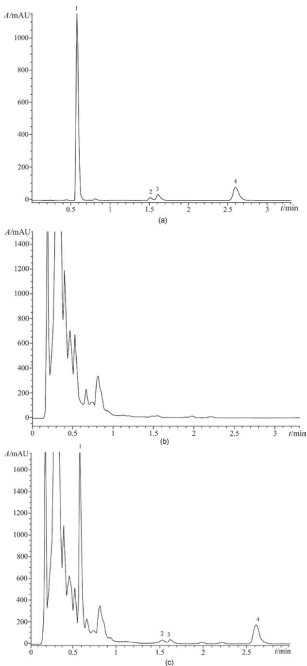
**Figure 3.** Chromatograms from standard mixture of atrazine (1), malathion (2), fenitrothion (3) and parathion (4) at the concentrations which correspond to MRLs (a), matrix blank (b) and samples of apple juice fortified at the concentration equal to MRL for each analyte (c).
