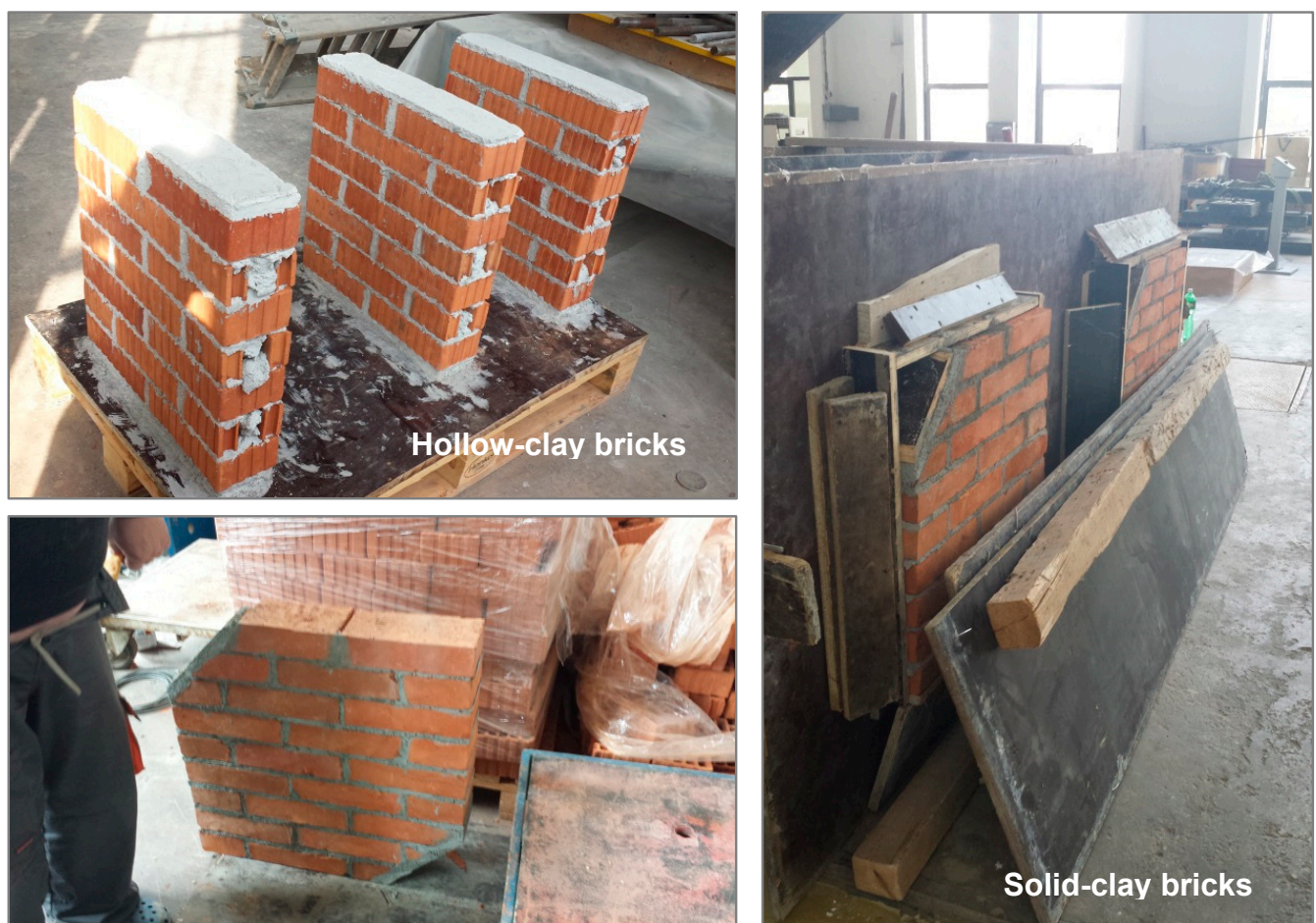
Figure 3. Wall elements for quasi-static testing [33].
