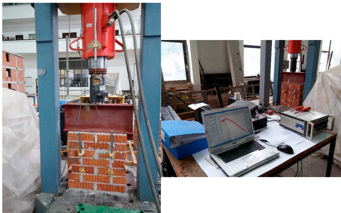
Figure 6. Experimental determination of compressive strength of hollow-clay masonry walls [33].
