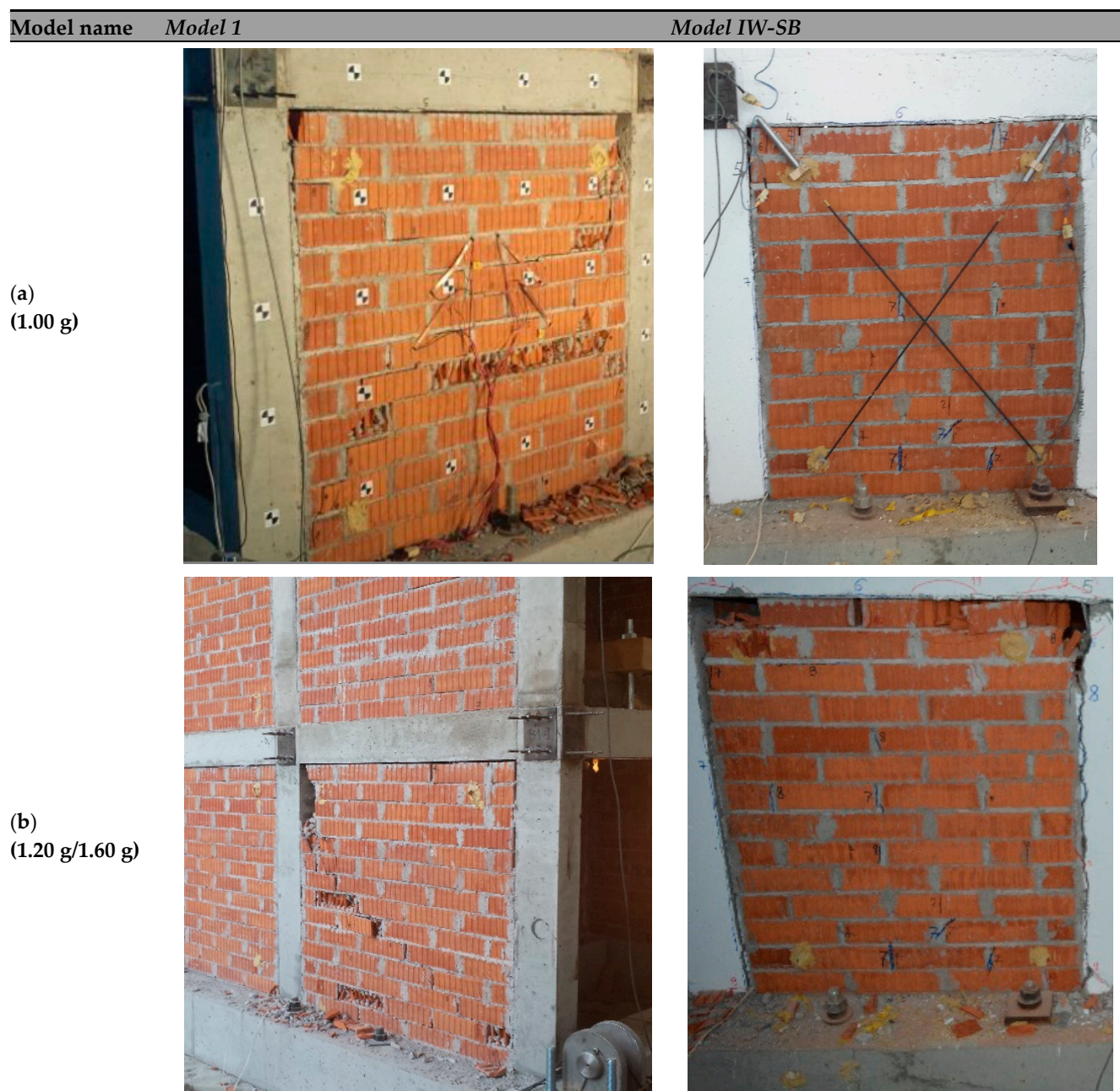
Figure 23. Observed in-plane damage (a) after 1.0 g and (b) after the final tests of 1.2 g/1.6 g, for Model 1 and Model IW-SB.
