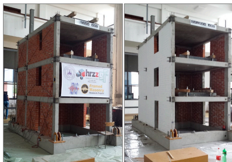
Figure 2. 3D view of Model 1 and Model 2 to a scale of 1:2.5 [33].
