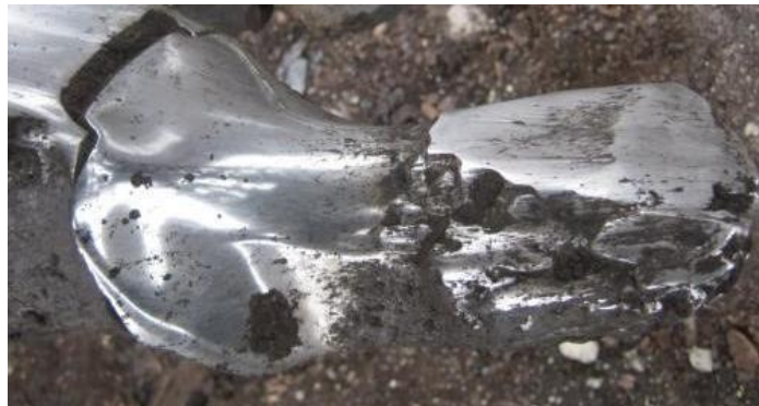
Figure 2: Decohesion of welded layers
