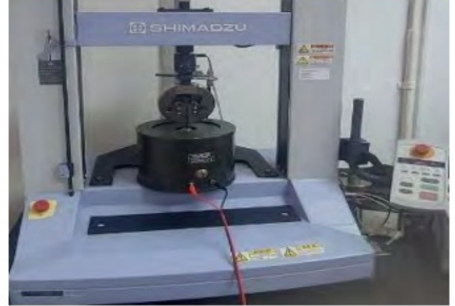
Figure 2. Experimental measuring on universal tensile testing machine
