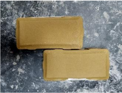
Fig. 4 Synthesized to 1127 °C end products ceramic pavers “yellow paving stone” type.
