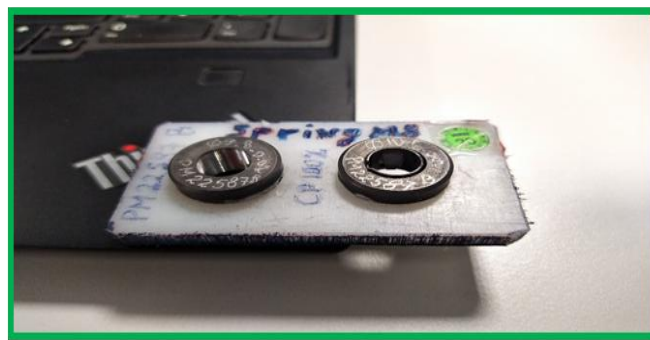
Fig. 4. OK and NOK spring test with the go-not-go gauge
