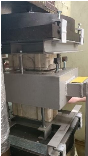
Fig. 3. View of the mounted die construction of the press facility for the main moulding.
