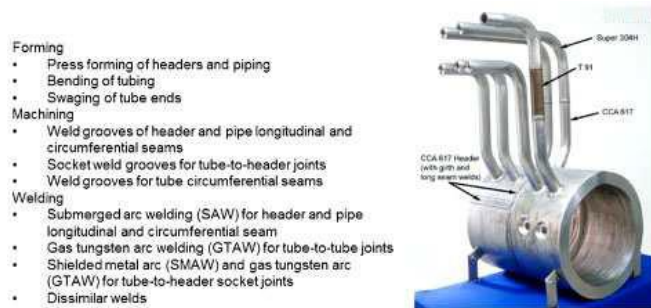
Fig. 1: Combination of materials, fabrication techniques and welding processes in fabrication of steam boiler [3]
