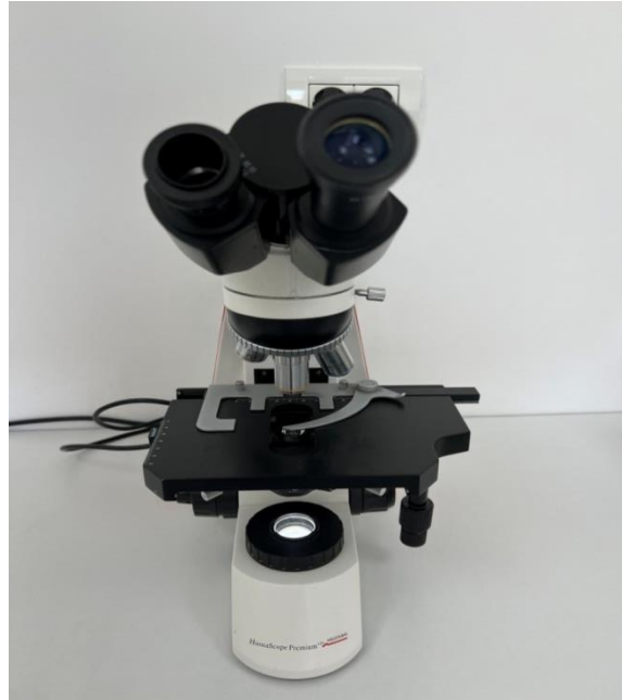
Figure 5: Optical microscope with LED illumination with premium optics (Humascop premium-Albimedica laboratory, 2025)
