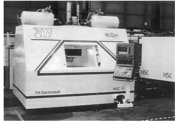
Fig. 3 High Speed Cutting CNC linear motor machine (HSC 11) at the Institute of Production Management, Technology and Machine Tools (PTW) at Technical University Darmstadt, Germany
