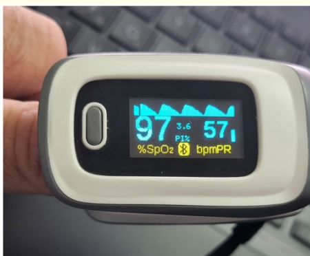
Figure 2: Commercial pulse oximeter with bluetooth connectivity: Displaying SpO 2 , heart rate, perfusion index, battery status, and real-time perfusion fluctuations on a spectral diagram.
