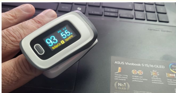
Figure 1: Commercial pulse oximeter with bluetooth connectivity: Displaying \text{SpO}_2 , heart rate, perfusion index, and battery status.
