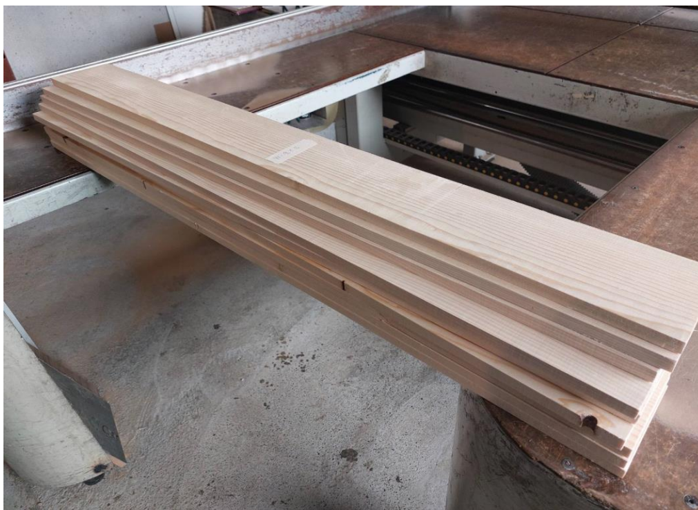
Слика 4. Prepared FIR/SPRUCE planks with a thickness of 15 mm
