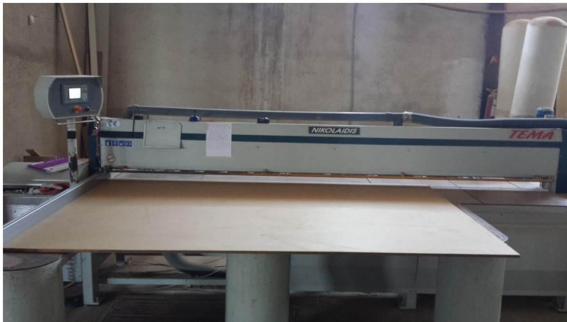
Figure 1. Panel circular saw with Greek origin: NIKOLAIDIS TEMA 3800
