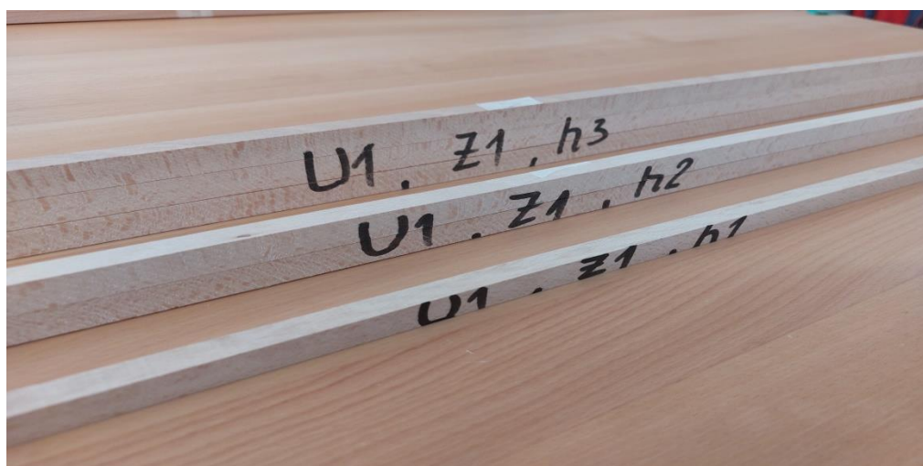
Figure 8. BEECH samples obtained at feed speed U_1=12 \text{mmmin}^{-1} , number of teeth Z_1=40 , for cutting height h_1=15\text{mm} , h_2=30\text{mm} and h_3=45\text{mm}
