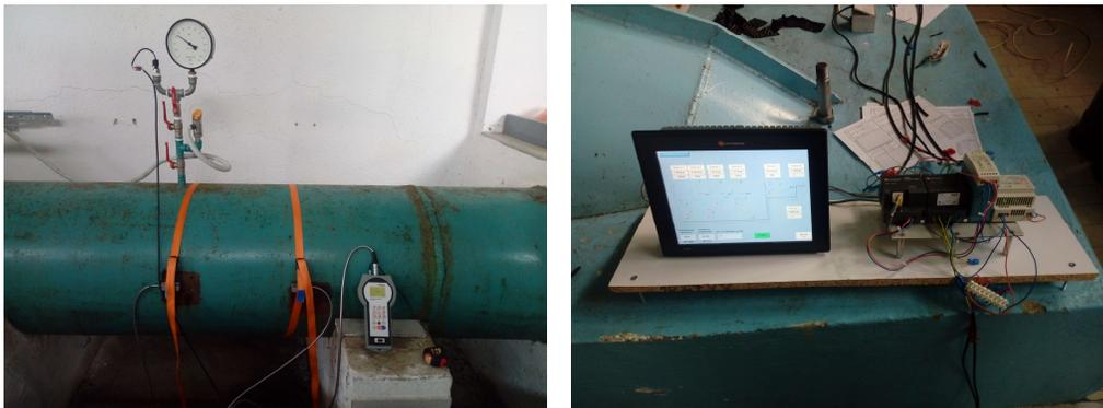
a) measuring pressure and discharge
