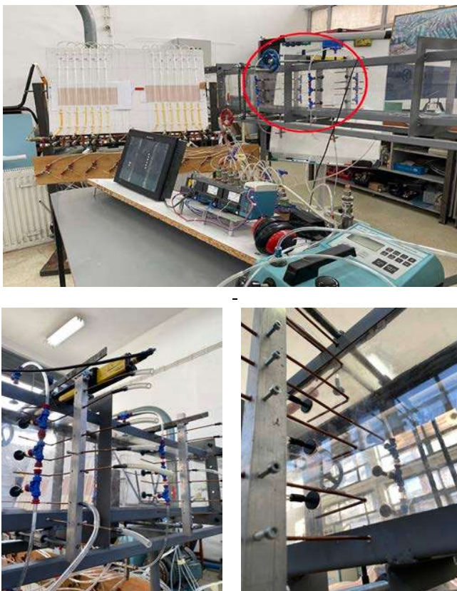
Figure 1. Experimental system for measurement of velocity: rectangular conduit with measuring sections and equipment
