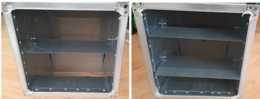
Figure 4. Elbow with one splitter vane (left) and two vanes (right)
