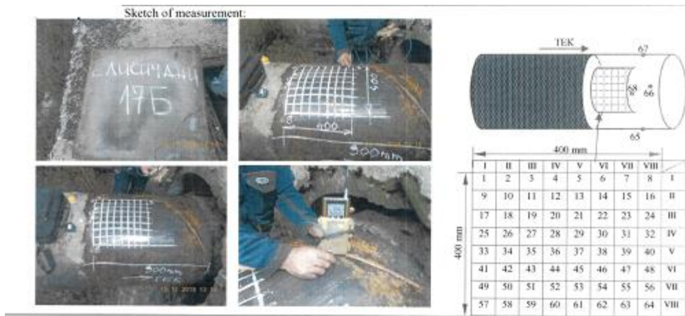
Figure 6. NDT test of pipeline
