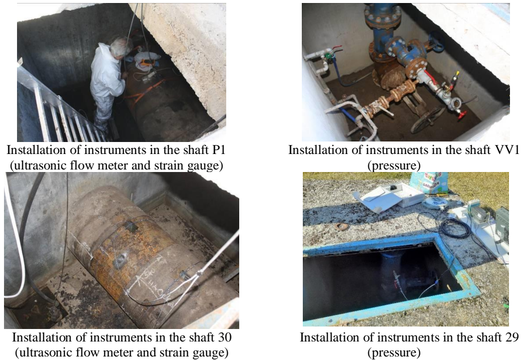
Figure 8. Measuring instrumentation for dynamic test of pipeline.
