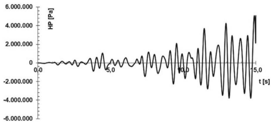
Fig. 14 The hydrodynamic pressure time history at node A for Case E2
