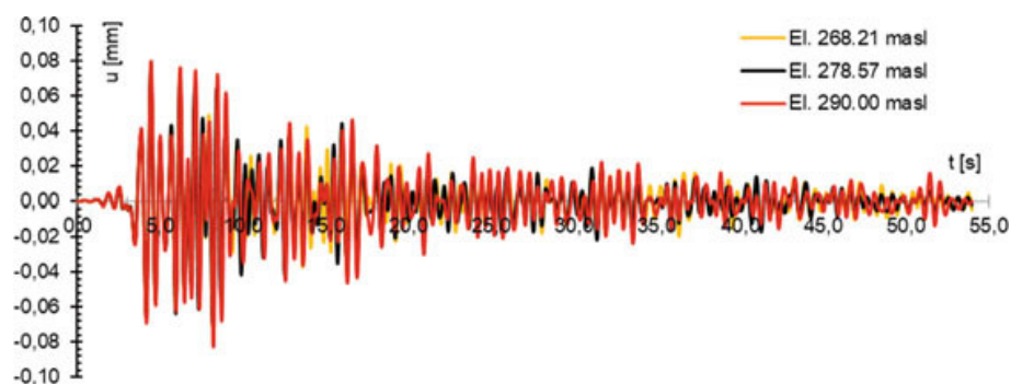
Fig. 9 The displacements time history of upstream node C for Case D1, D2 and D3
