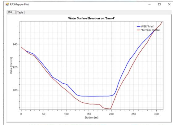
Figure 21. Water surface level at profile 00 – downstream of TSF Sasa 4, for scenario 2
