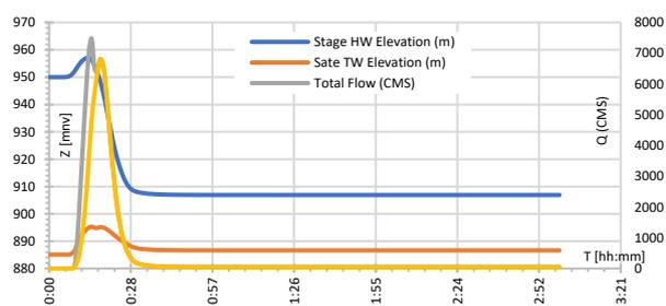
Figure 12. Hydrograph of water level and flood wave in the profile of TSF Sasa 3-2, for scenario 2
