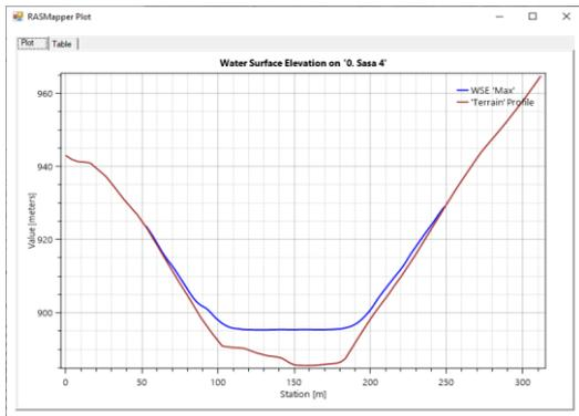
Figure 14. Water surface level at profile 00 – downstream of TSF Sasa 4, for scenario 1
