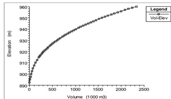
Figure 6. Volume – elevation curve for Sasa 4 TSF
