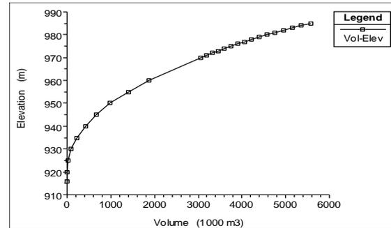
Figure 5. Volume – elevation curve for Sasa 3-2 TSF
