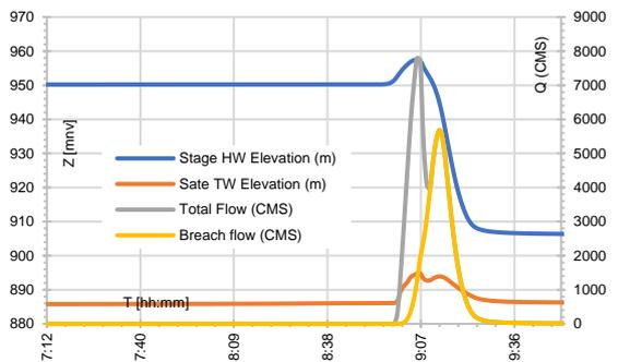
Figure 20. Hydrograph of water level and flood wave in the profile of TSF Sasa 4, for scenario 2
