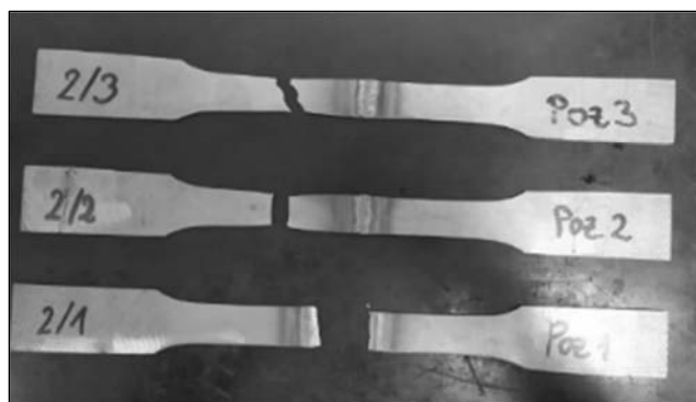
Figure 13. Tensile tested specimens from sample 2
