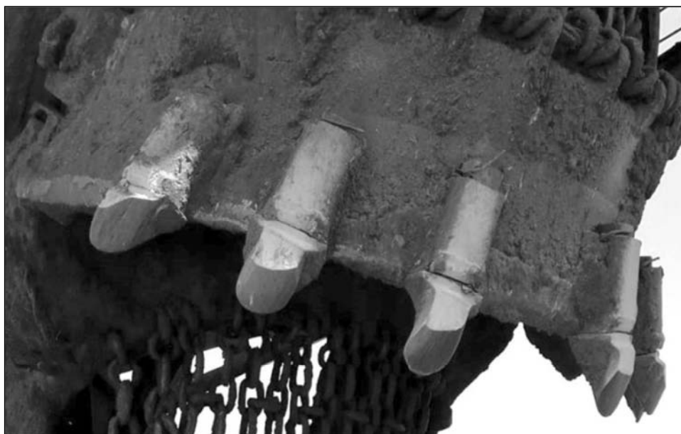
Figure 6. Influence of tooth position on degree of abrasion in SRS 2000 rotor excavator
