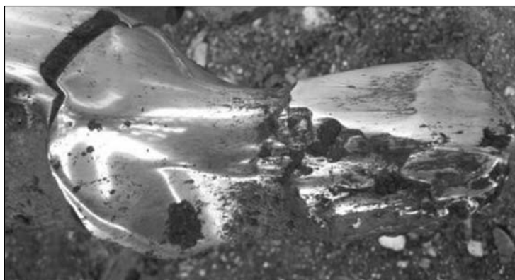
Figure 2. Delamination of hardfaced layers
