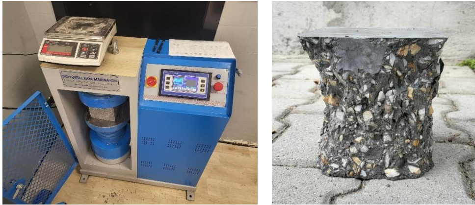
Fig. 4. Testing the strength of the concrete
