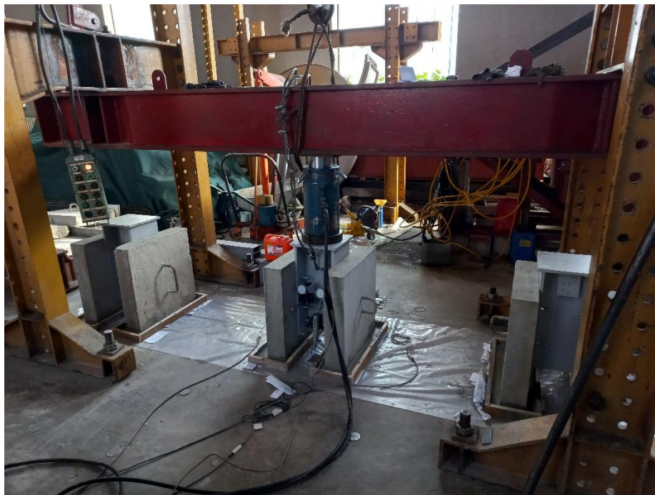
Fig. 6. Disposition of the loading and the measuring equipment in the University laboratory
