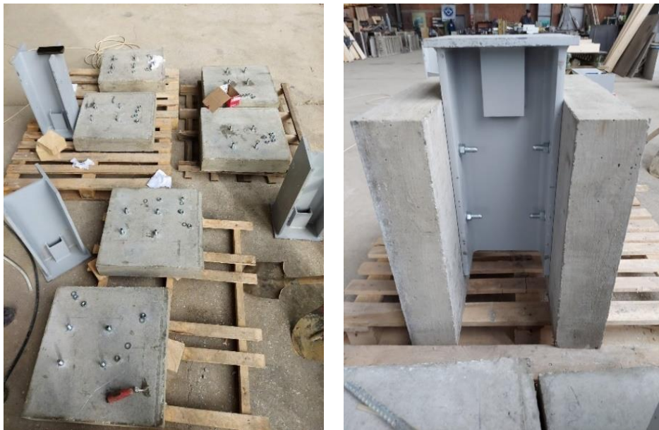
Fig. 3. Embedding of the concrete specimens with the steel beams and the anchor bolts
