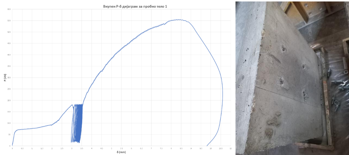
Fig. 8. P- \delta Diagram until force failure appears and the visible failure in the test subject 1
