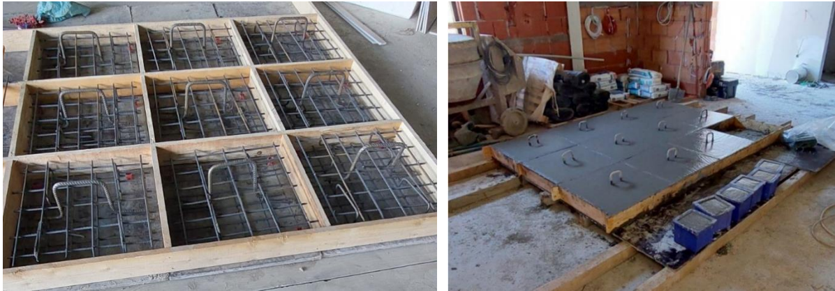
Fig. 2. Casting of the concrete for the modified testing specimen
