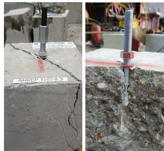
Figure 16. Failure of anchor type 7 and 8
