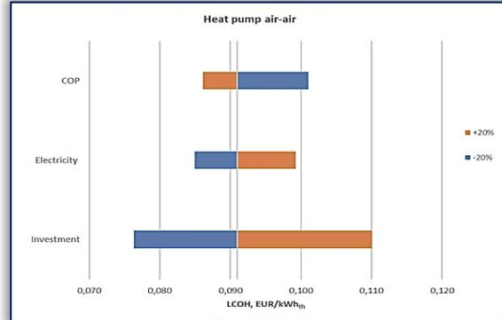
Figure 4. Sensitivity analysis for heat pump air–air LCOH – Scenario 1
