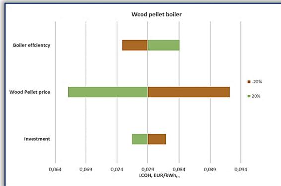
Figure 6. Sensitivity analysis for LCOH wood pellet boiler – Scenario 1
