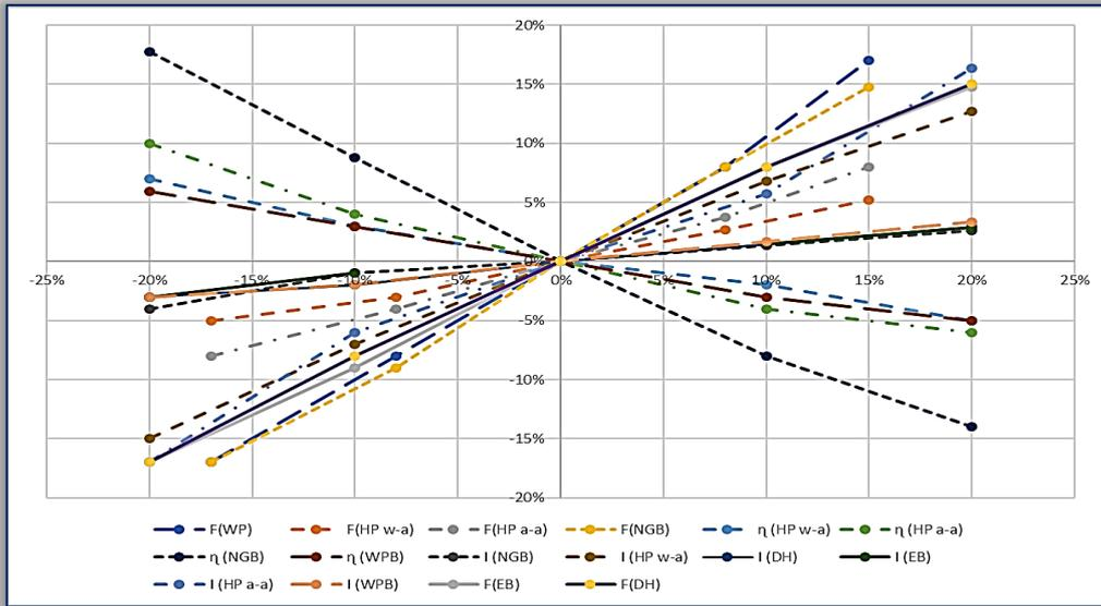
Figure 9. Change in LCOH relative to reference case as a function of I – CAPEX, F – fuel,  $\eta$  – thermal efficiency
