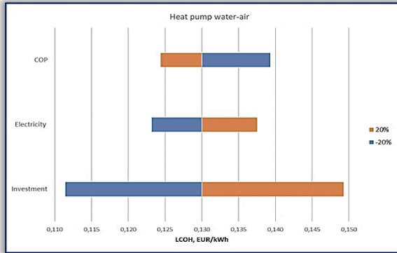
Figure 3. Sensitivity analysis for heat pump water–air LCOH – Scenario 1
