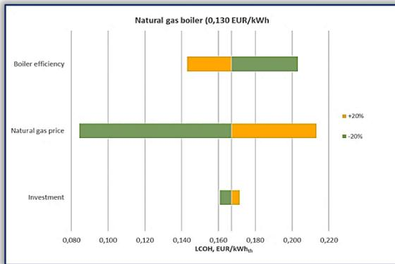
Figure 5. Sensitivity analysis for LCOH natural gas boiler – Scenario 1
