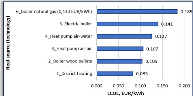
Figure 10. LCOE for heating, cooling and DHW
