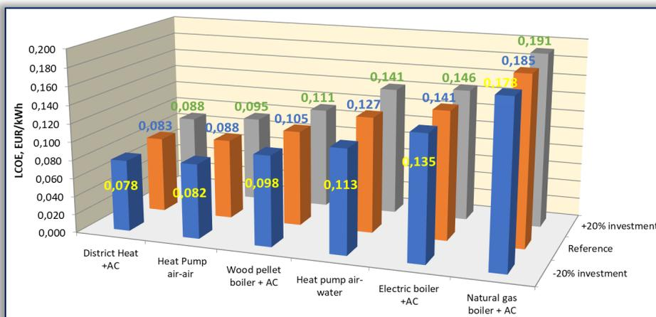
Figure 11. Sensitivity analysis for the LCOE with investment change, for systems providing heating, cooling and DHW
