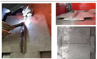
Figure 2.1 Pre-welding preparation, welding, and deformation after welding of Sample 1
