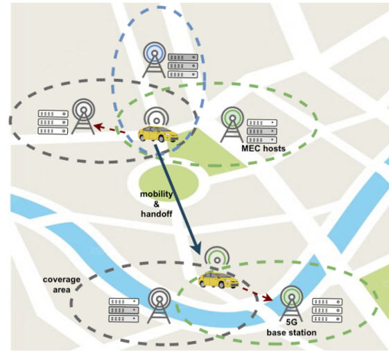
Fig. 1. 5G MEC architecture for the implementation of Internet of Vehicles.
