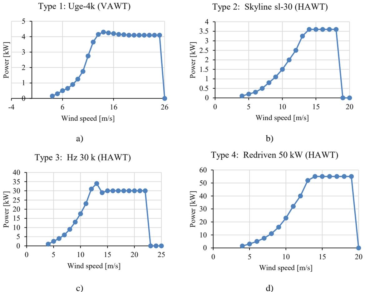
Figure 5 Power curves for four examined SWT according to data in Table 2
