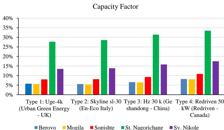
Figure 6 Calculated CF [%] for each SWT at the tested locations
