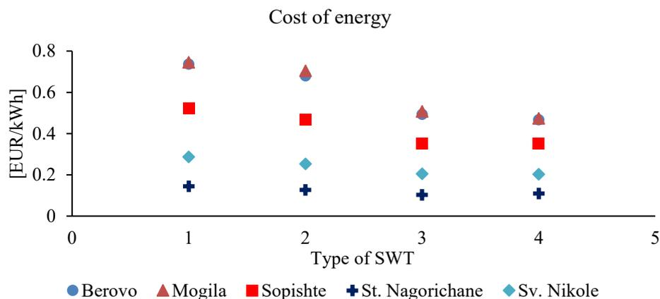
Figure 7 Unit Cost of energy production for each SWT at the tested locations
