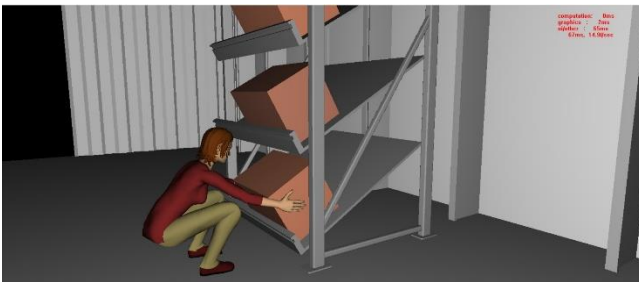
Fig. 9 Suggestion improvement – inclined shelves (30deg) for easier reach and grasp in challenging positions
