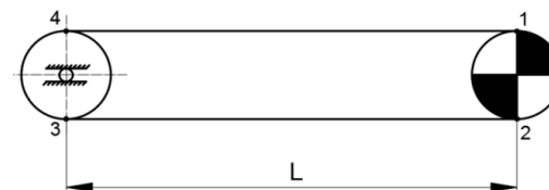
Figure 2. Schematic of the belt conveyor route
