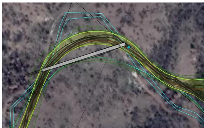
Figure 6. Maps satellite image for passability check with tire tracks of tractor and trailer
