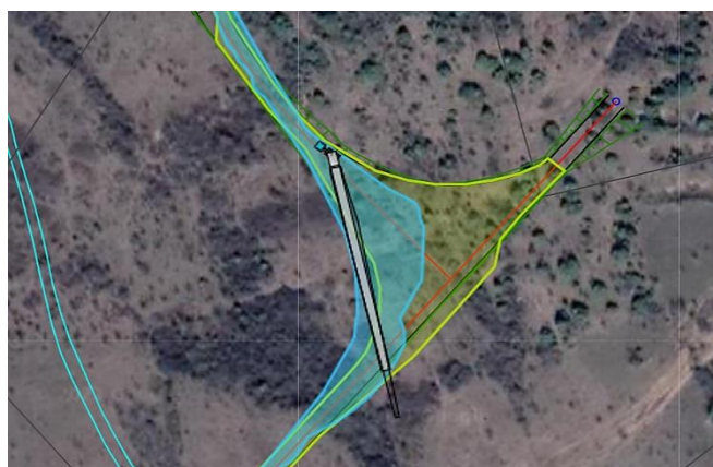
Figure 7. Maps satellite image for passability check with area covered by vehicle combination
