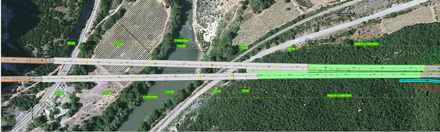
Figure 1. Horizontal layout, console bridge and reinforced earth
