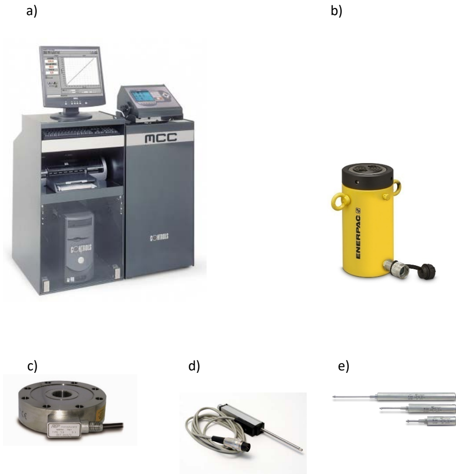
Fig. 4.27 Photo of items used for the experiments; a) Multifunctional Control Console (MCC 8), b) Hydraulic Cylinder, c) Force Transducer, d) Linear Potentiometer Transducer and e) Displacement Transducer
