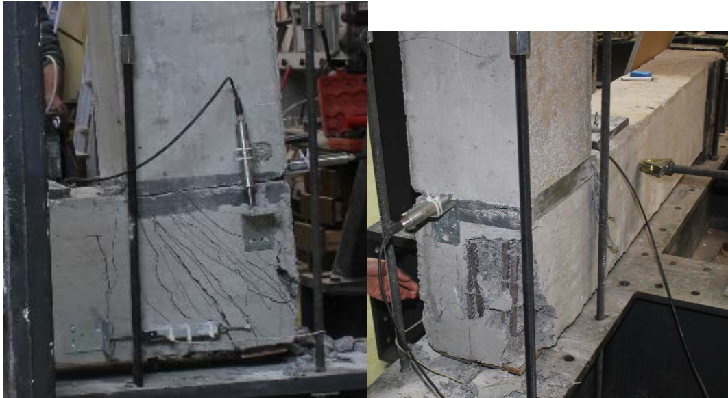
Fig. 4.44 Crack pattern of the specimen under the last loading cycle - photo from the experiment on specimen "S.3 V.D."
