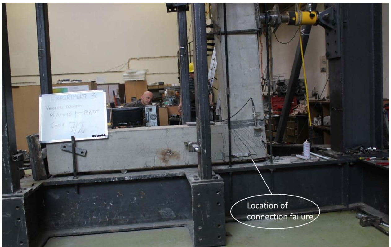
Fig.5.17 Crack distribution on specimen "S 3, V.D." after failure.
