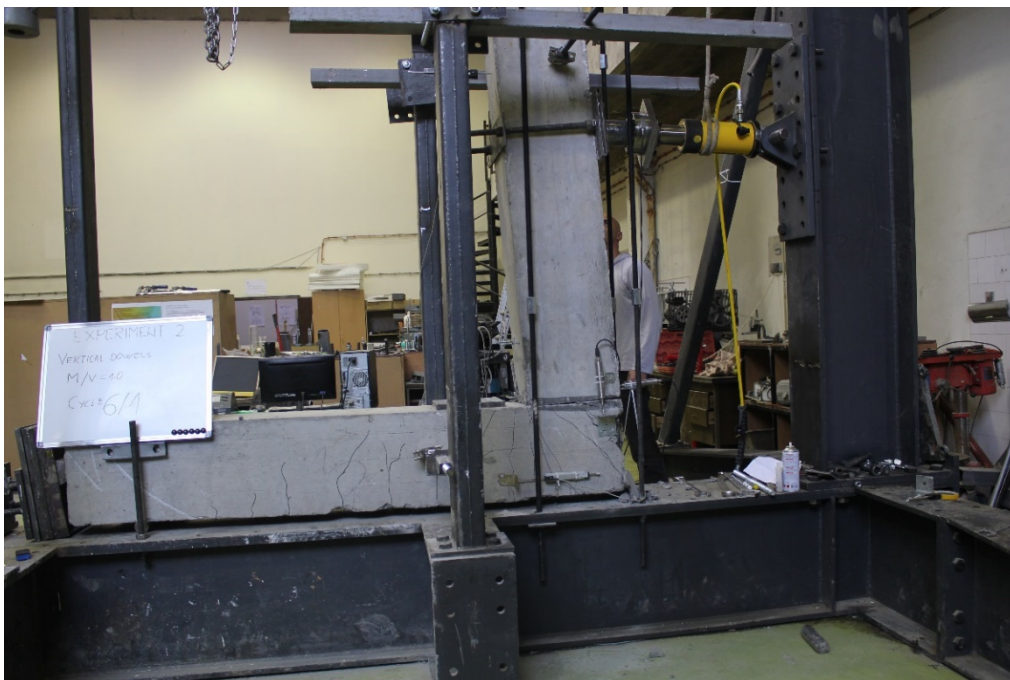
Fig. 4.38 Crack pattern of the specimen at the last loading cycle -photo from experiment of specimen "S.2 V.D."
