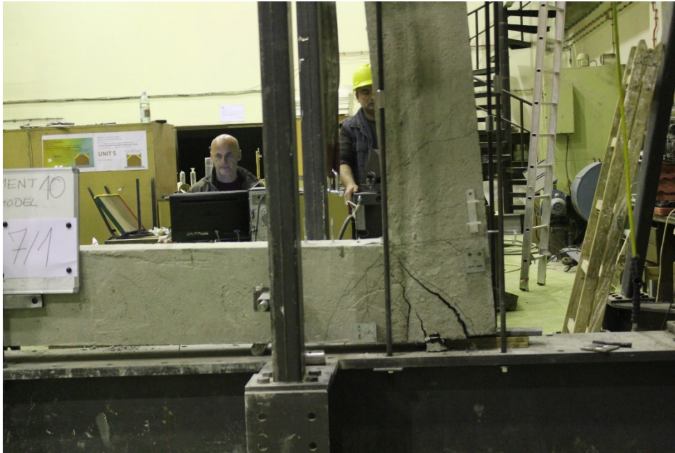
Fig. 4.81 Photo of the specimen after the last loading cycle applied on specimen "S.10 R.M."
