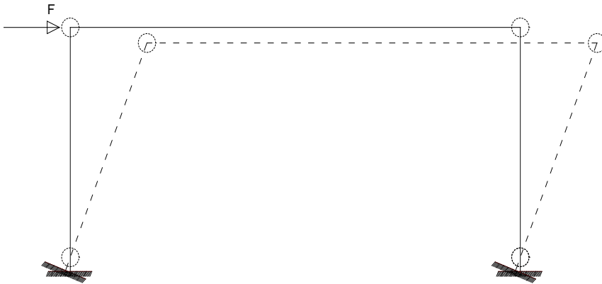
Fig. 2.17 Potential failure mechanism due to increase of displacement of a mechanically instable frame should plastic hinge is created as in fig. 2.16
