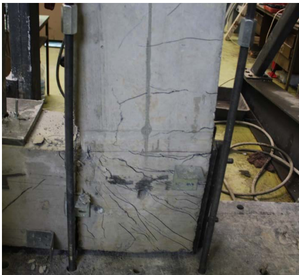
Fig. 4.78 Photo of the specimen after the last loading cycle applied on specimen "S.9 H.D."
