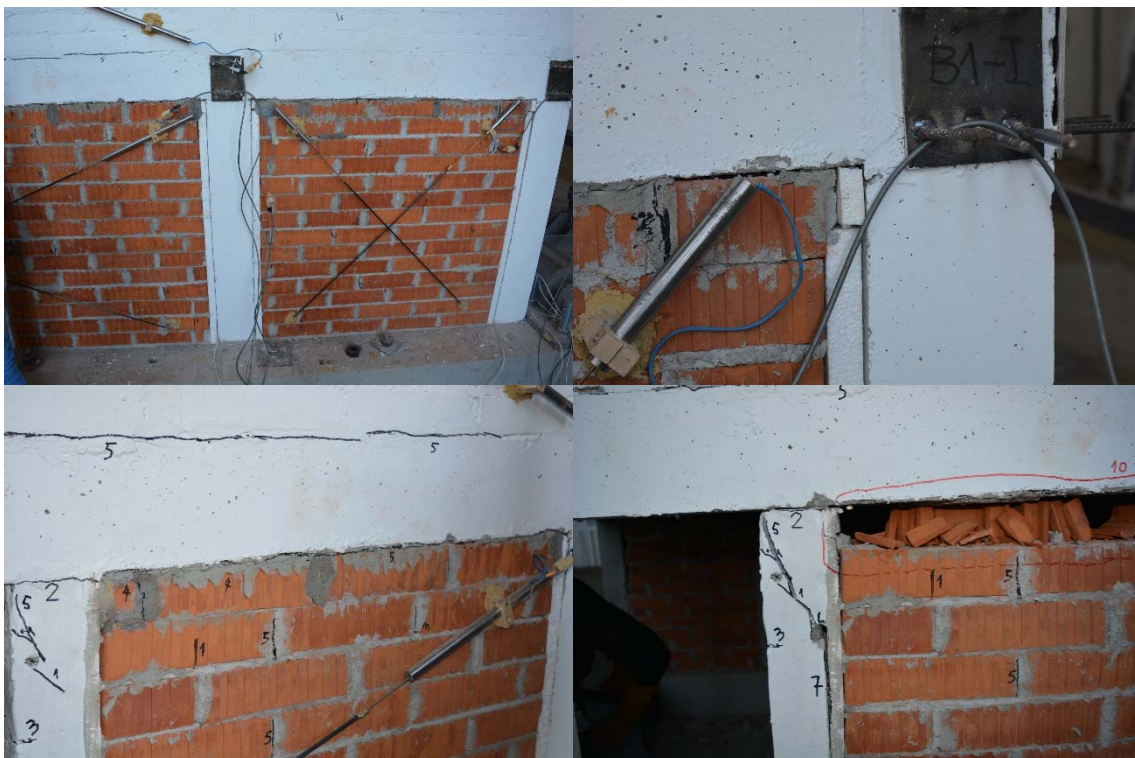
Figure 4.29 Damage to infill of the Model IW-SB, frame A – infill connection - first variant solution
