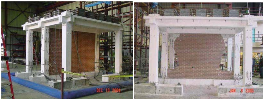
Figure 3. 8 Test structure and failure mode of infill panels after shake-table tests (Heshemi and Mosalam, 2006)
