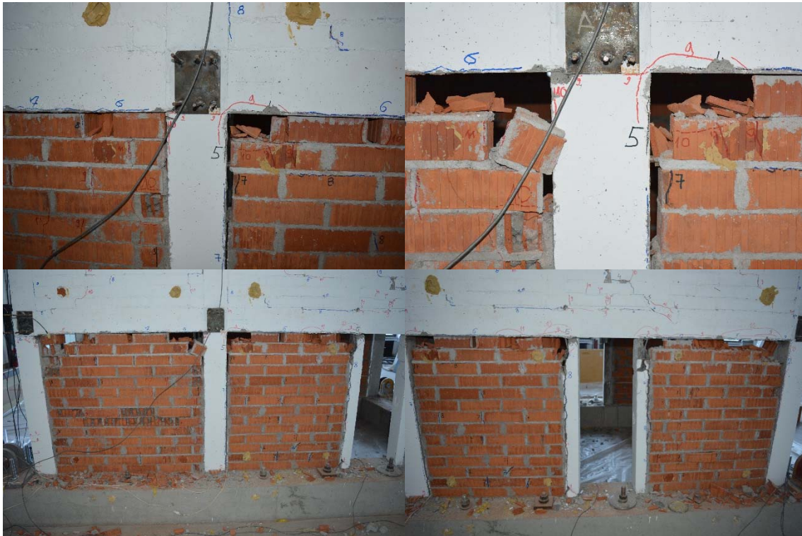
Figure 4.29 Damage to infill of the Model IW-SB, frame A – infill connection - first variant solution
