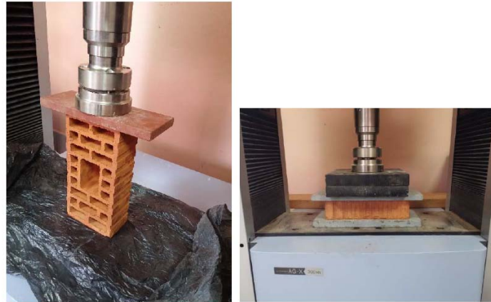
Figure 4.5 Experimental determination of compression strength of hollow-clay masonry units (Report IZIIS 2015-31)
