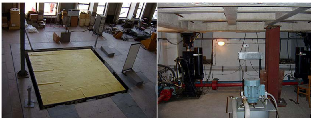
Figure 4.11 IZIIS' seismic shake table – top view (left), below the table (right)
