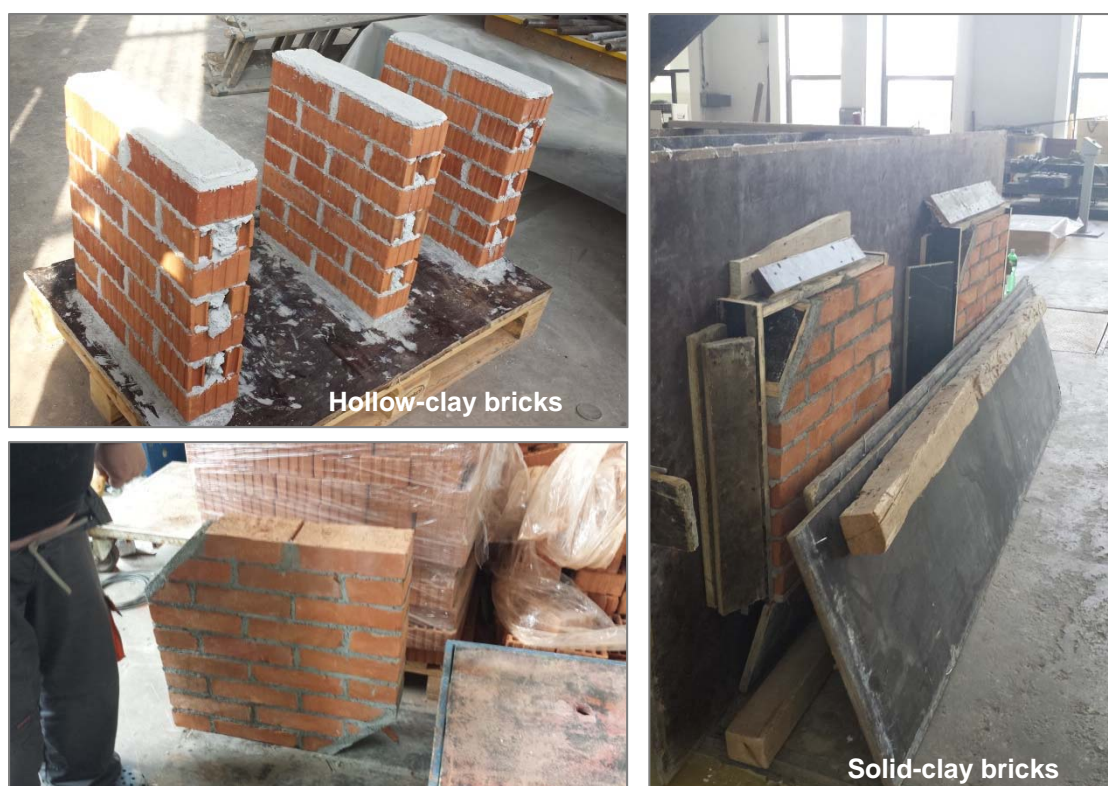
Figure 4.6 Wall elements for quasi-static testing (Report IZIIS 2015-31)
