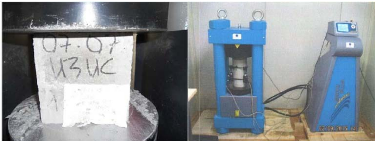
Figure 4.4 Experimental determination of concrete compressive strength and modulus of elasticity (Report IZIIS 2015-31)
