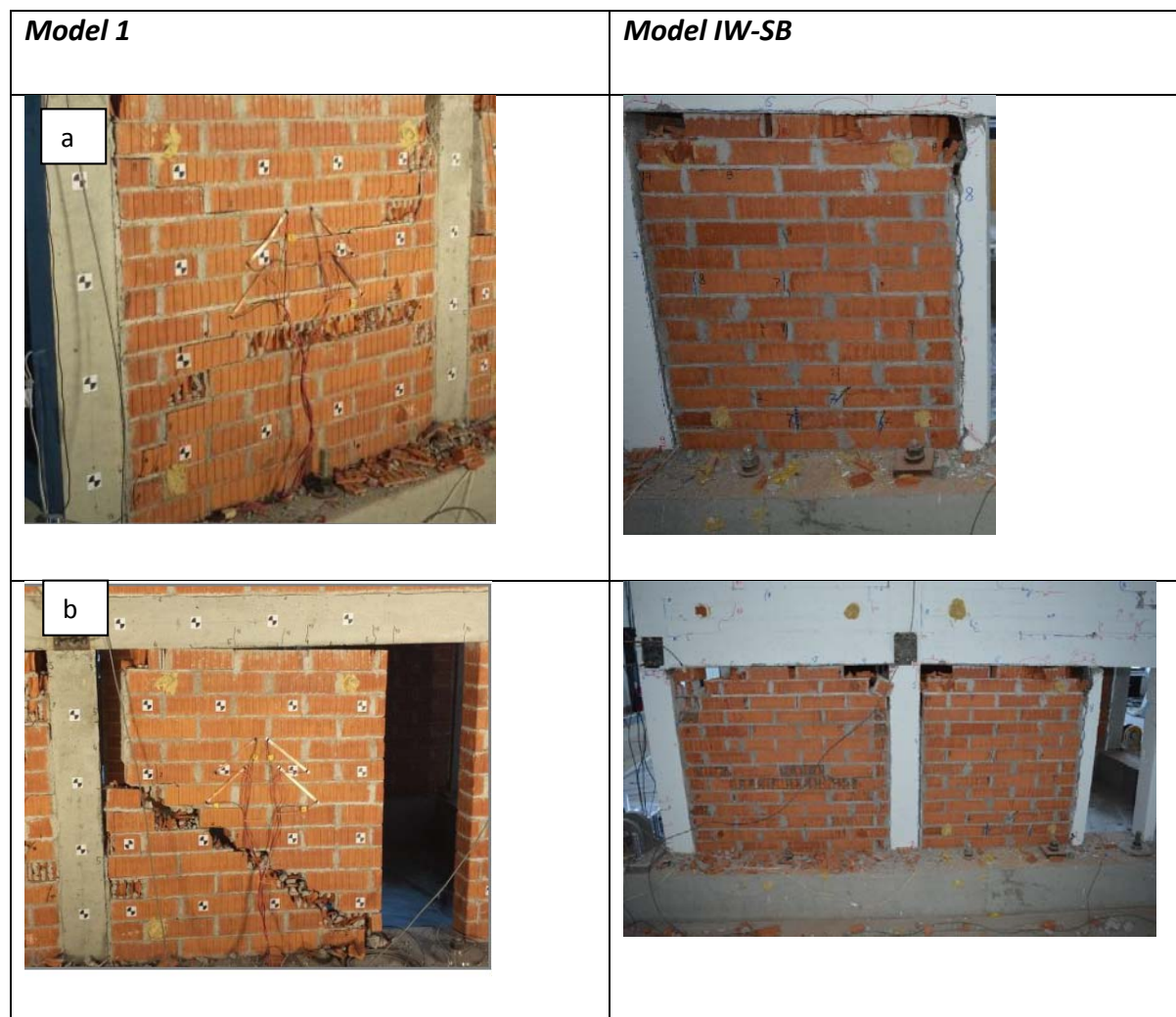
Figure 4.50 Observed in-plane damage a) after 0.4g and b) after the final tests of 1.2 g/1.6g, for Model 1 and Model IW-SB
