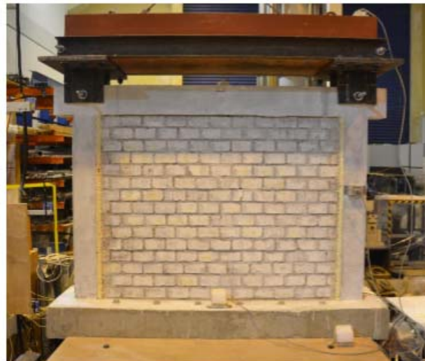
Figure 3. 11 Shaking table tests performed by Zhang (2015)
