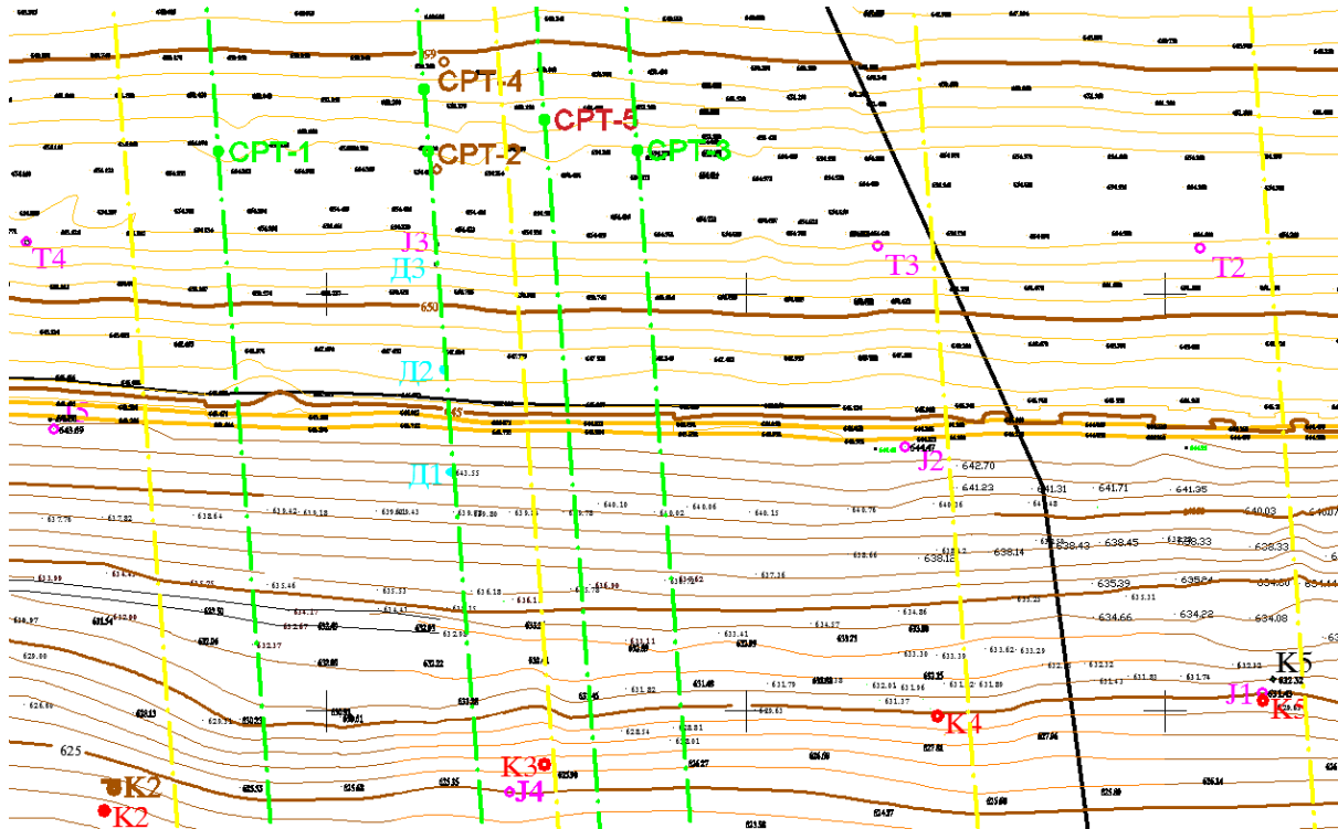
Figure 1: Layout of inclinometers J1, J2, J3, J4 and J5 and geodetic surveying points T 2 , T 3 and T 4 .
