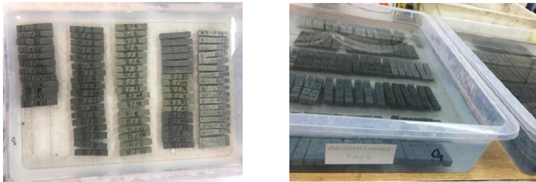
Figure 3: Curing of specimens
