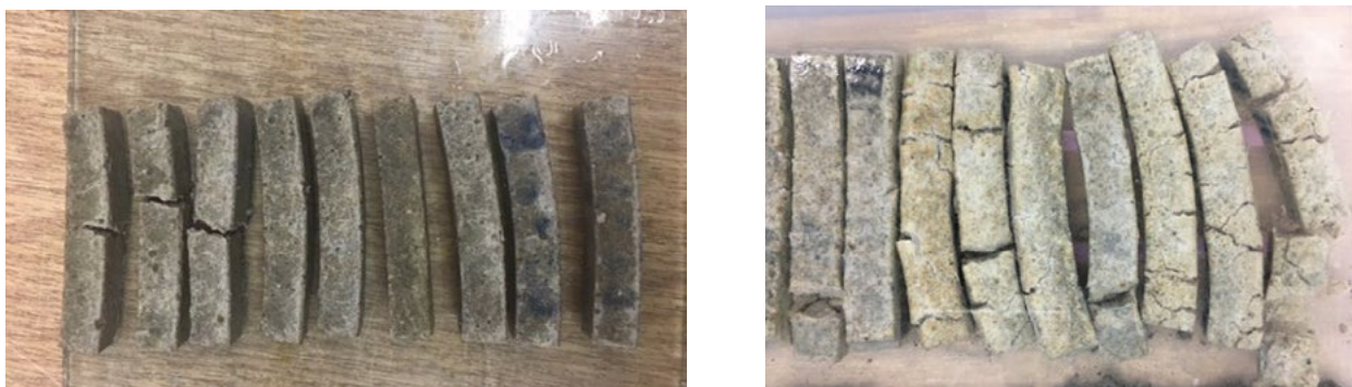
Figure 5: Deformed prisms made of pure cement 18 and 90 days after immersion in 4.4% \text{Na}_2\text{SO}_4
