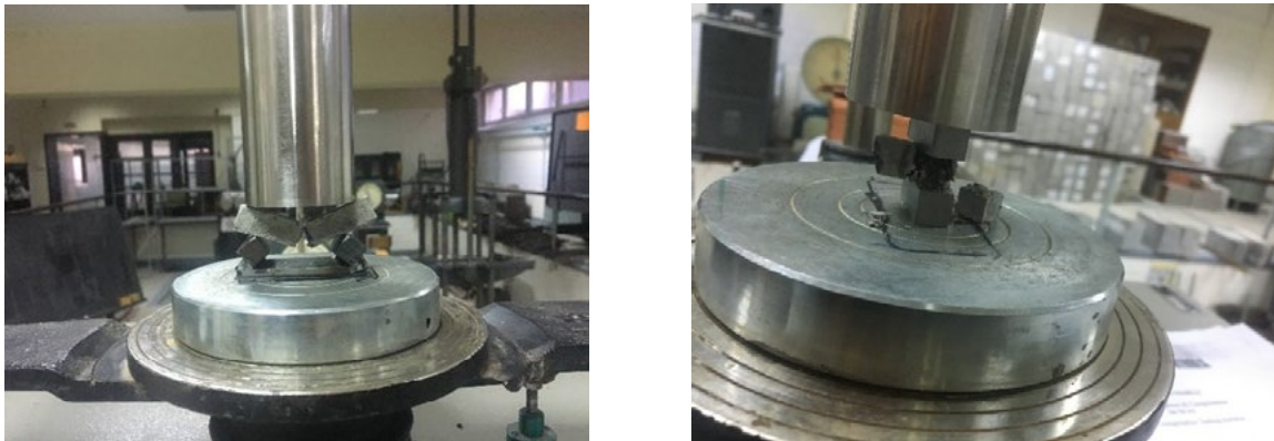
Figure 4: Testing of flexural and compressive strength
