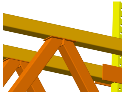
(b) Detail of the K bracing
