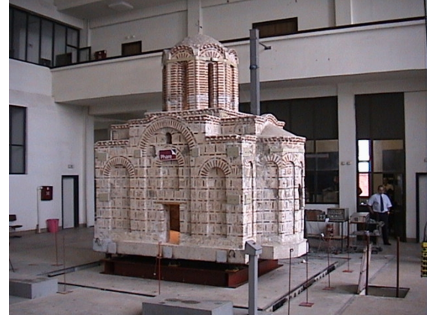
(b) St. Nikita church model on a shaking table
