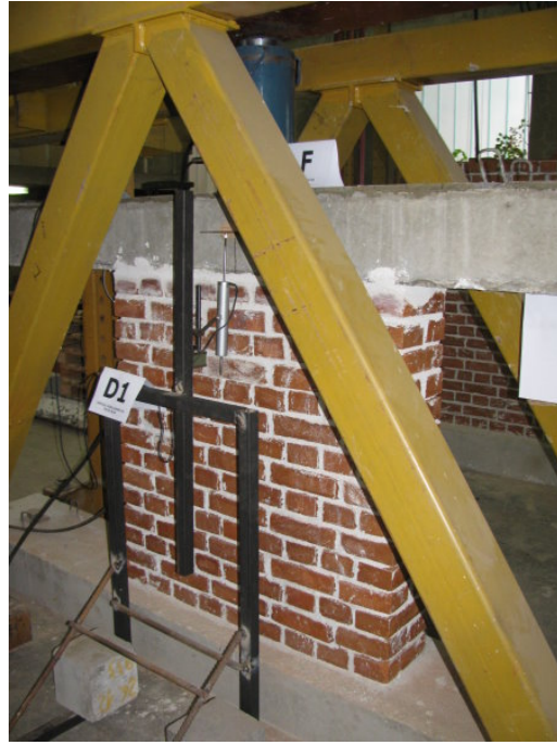
Figure 60: Test set-up for compressive strength of masonry
