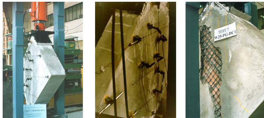
(b) Tests on strengthened masonry wallets with geogrids
