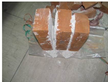
(b) A.1 type of failure obtained in the triplet specimen
