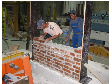
(b) Levelling the courses in both orthogonal directions
