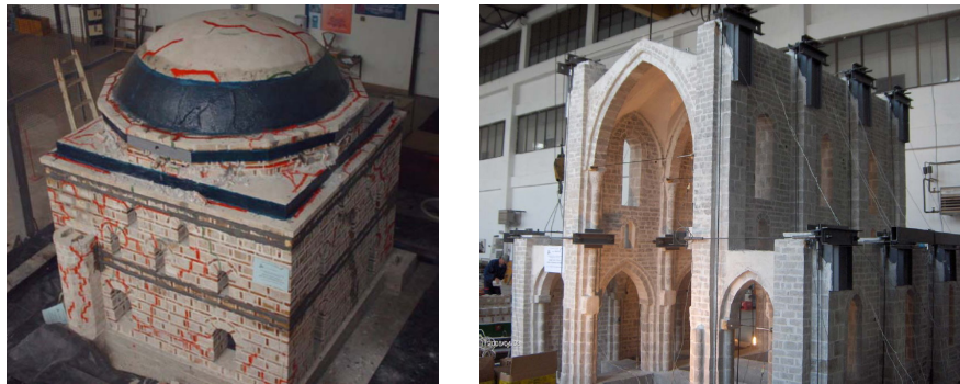
(a) Strengthened large scale model of Mustapha Pasha Mosque with C-FRP elements (b) Strengthened large scale model of Fossanova Cathedral with FRP cables
