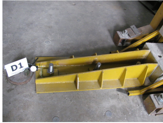
Figure 81: Clamping device for the bottom RC beam
