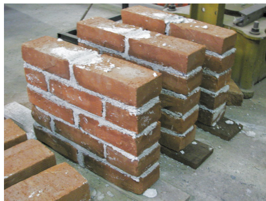
Figure 65: Wallets UMWC-2 for testing masonry compressive strength
