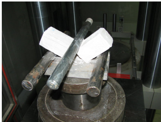
Figure 53: Typical tensile flexural failure mode of mortar specimen
