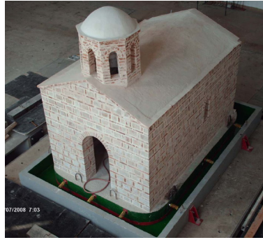
(a) The model of St. Nikola church with base isolating ALSC system
