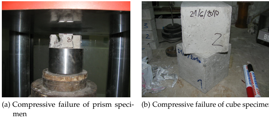
Figure 58: Compressive failure modes of concrete
