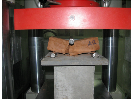
Figure 49: Tensile flexural failure mode of brick unit
