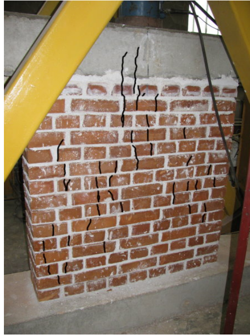
Figure 64: Failure mode at the end of the compressive test on wallet UMWC-1
