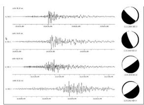
Figure 3: The waveforms of the vertical components of the strongest earthquakes recorded at the station in Skopje (SKO) and the corresponding P-nodal solutions (beach balls).
