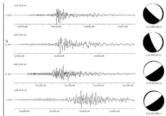
**Figure 3:** The waveforms of the vertical components of the strongest earthquakes recorded at the station in Skopje (SKO) and the corresponding P-nodal solutions (beach balls).
