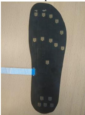
Figure 2. Insole Showing Array of Sensor Terminals
