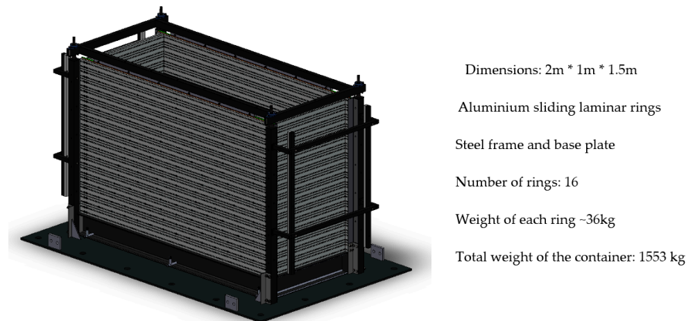
Figure 3. The 3D layout and main characteristics of the laminar container.
