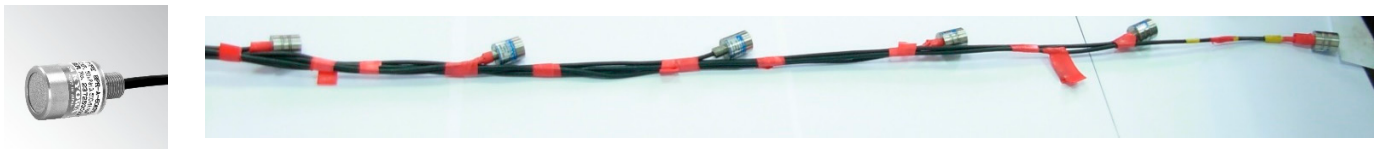
Figure 10. PWP transducer (left) and PWP line prepared for the sand model (right).
