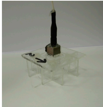
Figure 8. Accelerometer that is pressed into the soil.
