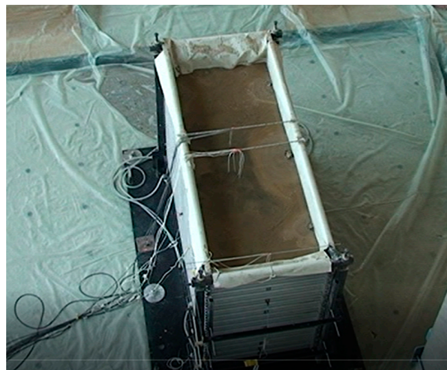
Figure 18. Visible manifestation of sand boils after liquefaction initiation (test No. 1).
