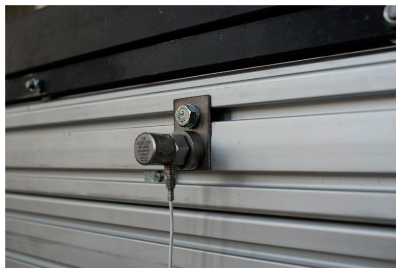
Figure 7. Accelerometer placed on the laminar ring.
