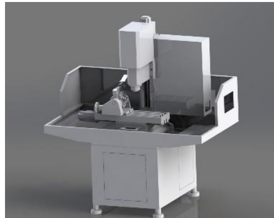
Fig. 2 A rendered view of the CNC machine assembly
