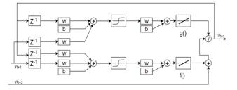
Figure 2. NARMA-L2 neuro-controller structure [13]
