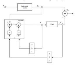
Figure 1. Block diagram of the NARMA-L2 controller [13]
