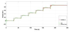
Figure 7. Comparison of the responses given by PID controller and neuro-controller
