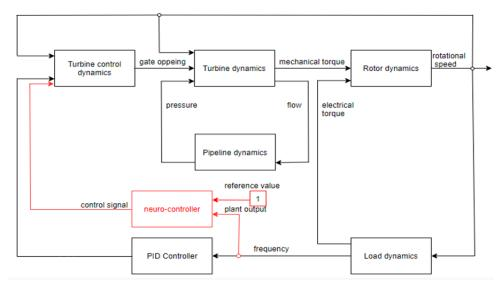
Figure 3. Block diagram of a hydropower plant [2] (amended by authors)
