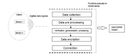
Figure 3. Display of processes running on sensor data
