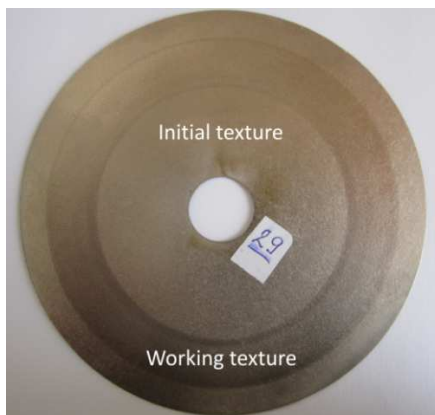
Fig. 6. Optical image of the initial and working texture on the tested coated discs (coating Ni-SiC HT )
