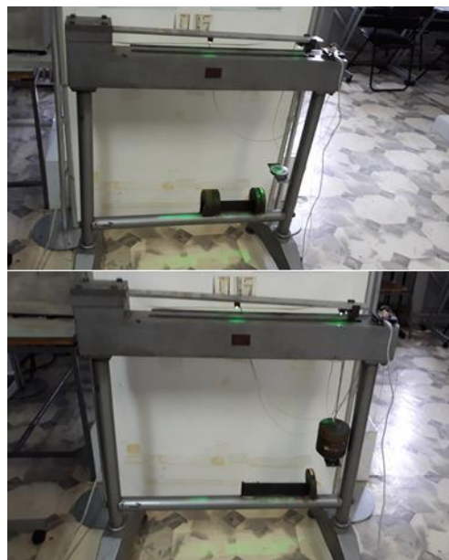
Figure 5. Photo of experimental set with unloaded and loaded beam
