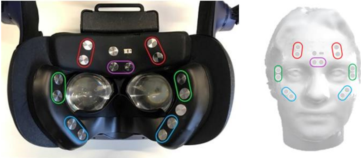
Figure 1. Left: The emteqPRO multi-sensor mask, showing the EMG channels: frontalis (in red), orbicularis (in green), zygomaticus (in blue) and corrugator (in purple). Right: The locations of the sensors mapped on the face.
