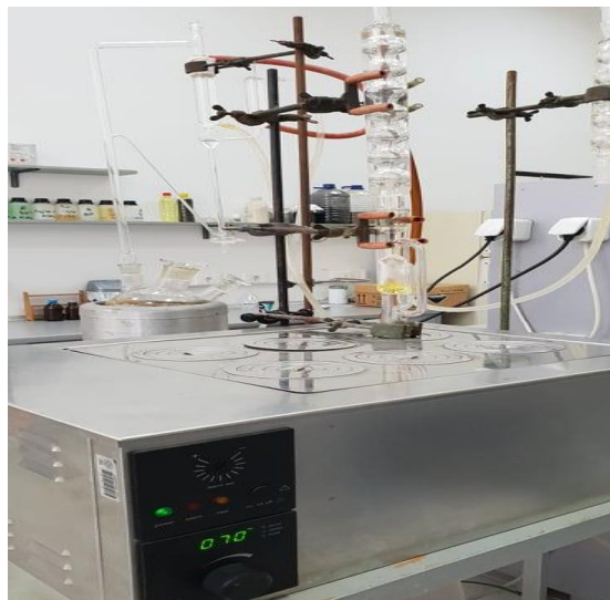
Figure 5 Complete Soxhlet apparatus
