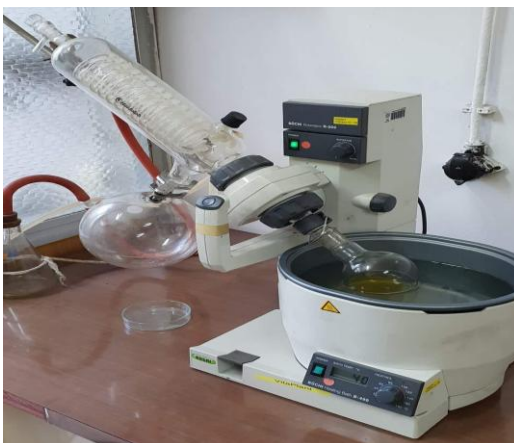
Figure 7. The appearance of rotavapor
