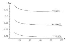
Fig. 6: Ass depending on the number of nodes when  $\rho$ =const=50 node per km2
