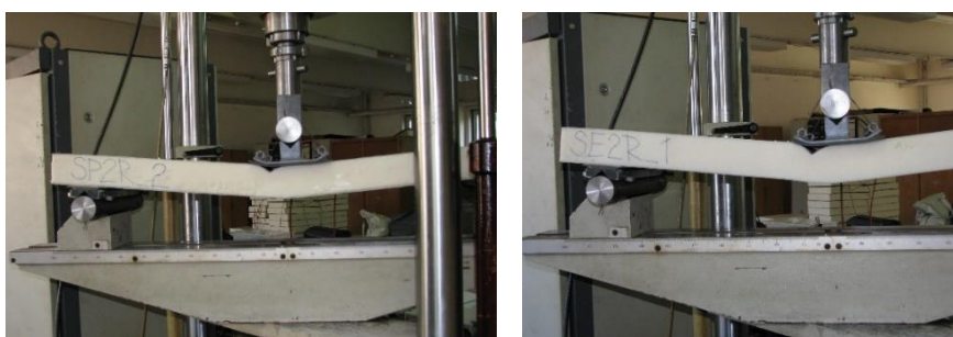
Figure 14: Fracture of the sandwich panels SP2R and SE2R subjected on three points bending
