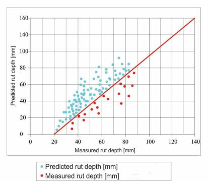
**Fig. 3**. Relation between the envisaged and the measured rutting depth in the non-calibrated HDM model (Default model) Source: Own research
