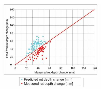
**Fig.. 4**. Relation between the envisaged and measured change of the rutting depth in the calibrated HDM model. Source: Own research
