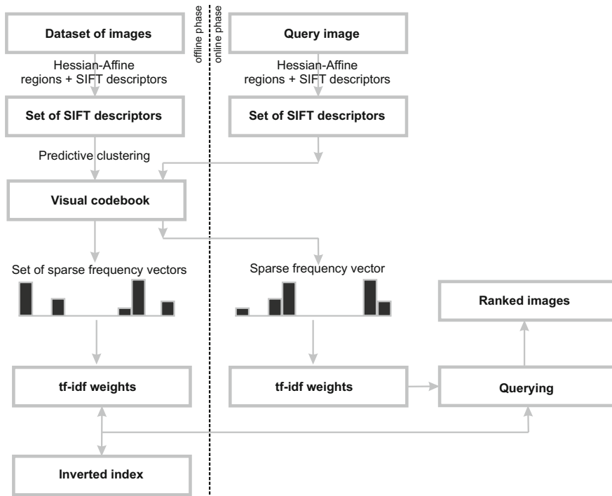
Fig. 2. Architecture of the proposed system for fast and scalable image retrieval based on predictive clustering trees
