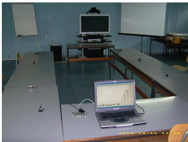
Fig. 4. Experimental setup with seven MicaZ motes and one clusterhead mote connected to a laptop.
