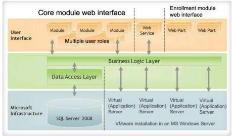
Fig. 3 Software architecture of the system
